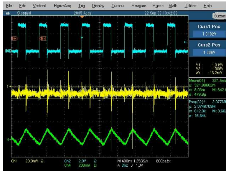
Figure 15. L=GLK2510P-2R2M, C=Ceramic 10 \mu F 0603 X5R YAGEO (Ripple 13.2mV)
