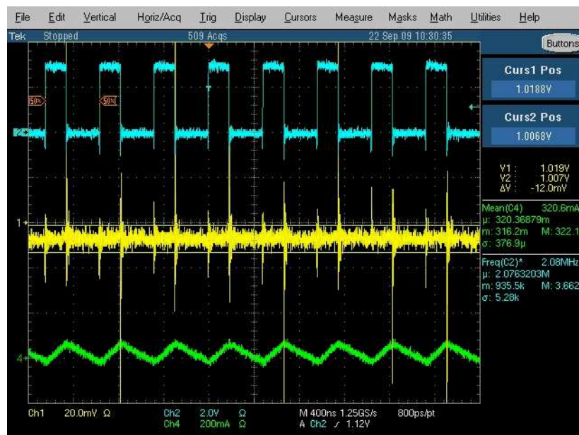
Figure 16. L=GLK2510P-4R7M, C=Ceramic 4.7 \mu F 0805 X5R TDK (Ripple 12mV)
