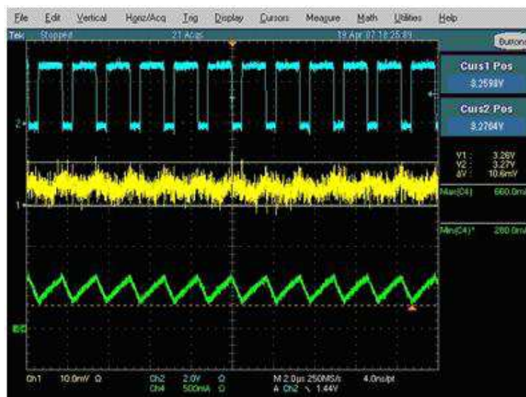
Figure 13. Ceramic 10 \mu F 0603 (X5R) (Good)
