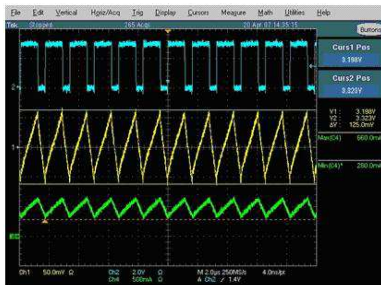
Figure 20. Electrolytic 100 \mu F (Ripple Too High)
