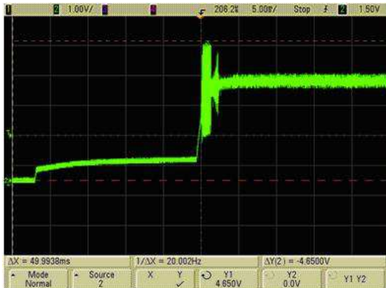
Figure 12. Input Voltage Overshoot >4V (Bad)
